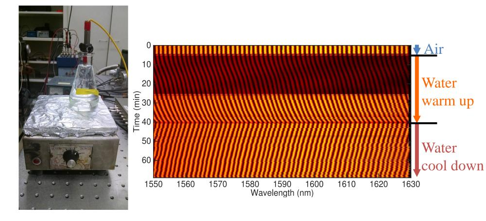
If the temperature of the test chamber can be raised in a controlled manner, a swept laser source is not needed to measure the temperature. Instead sweeping the temperature while keeping track of the reflected power at a single wavelength is enough to measure the relationship of temperature to reflected power. This calibration can be used to determine the temperature with a fixed wavelength laser source.
