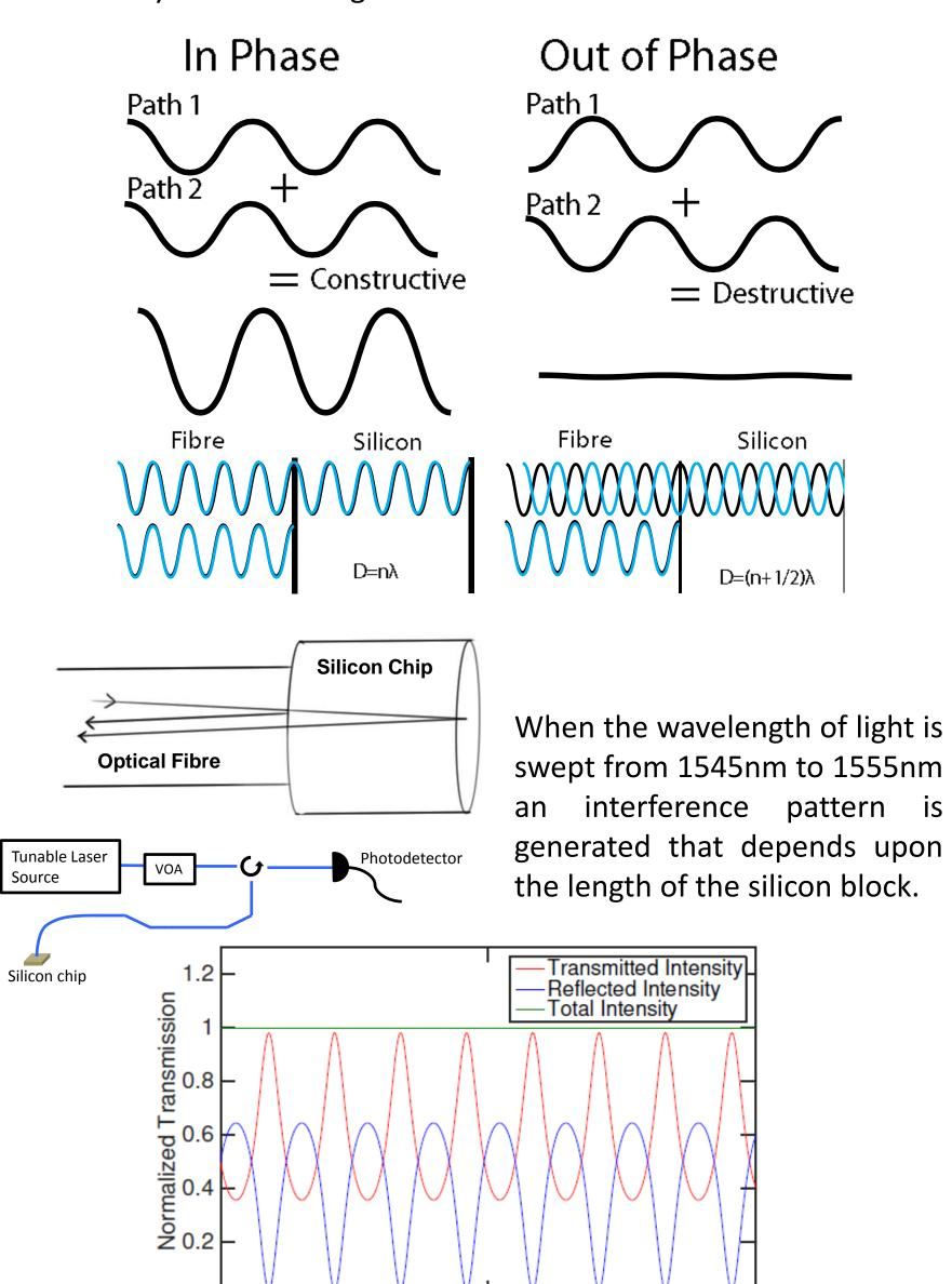
As the silicon block is heated the length increases which shifts the interference pattern. This shift is shown below as the sensor was heated to 100°C in water and then cooled back to room temperature.
