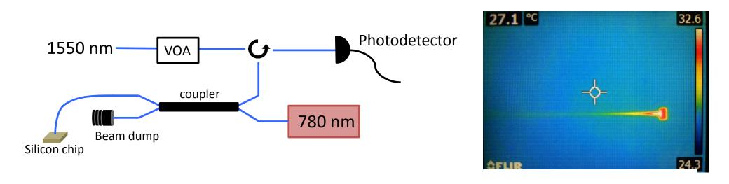
The optical absorption of silicon is uniquely suited for this application as silicon is opaque and can be heated by lasers below 900nm in wavelength and it is transparent and can be measured by light with a wavelength above 1500nm.
